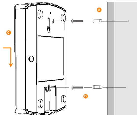
4. Place the AP onto the mounting screws so that the screw heads enter the keyholes on the AP enclosure (C), and gently
