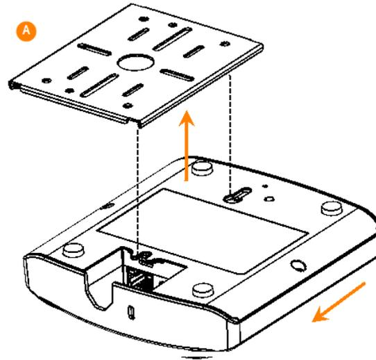
3. Insert the two studs on the secure mounting bracket (A) into the keyholes on the bottom of the AP.
